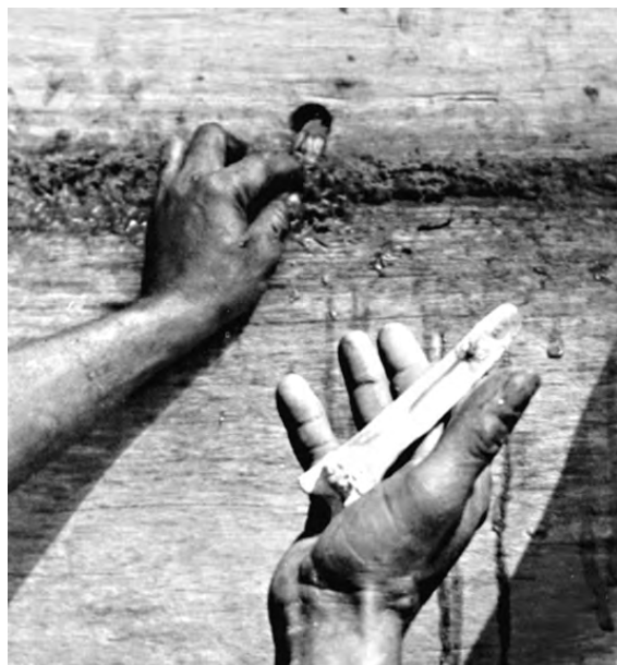
Dimsol tool used to caulk the holes with dim.
