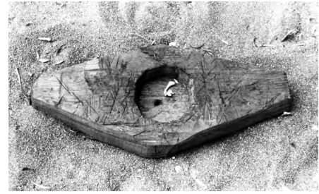
The mast step, the purarang, lies on the base of the hull.
